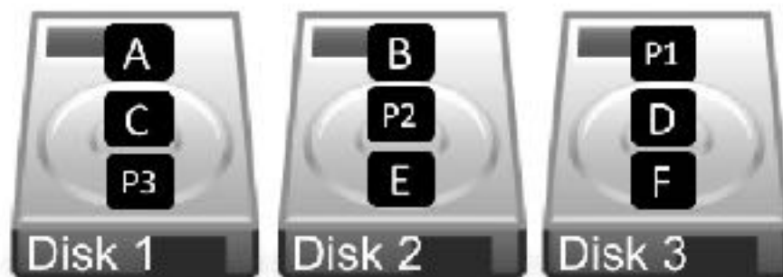
Figure 123: RAID 5 – Multiple drives with parity information
