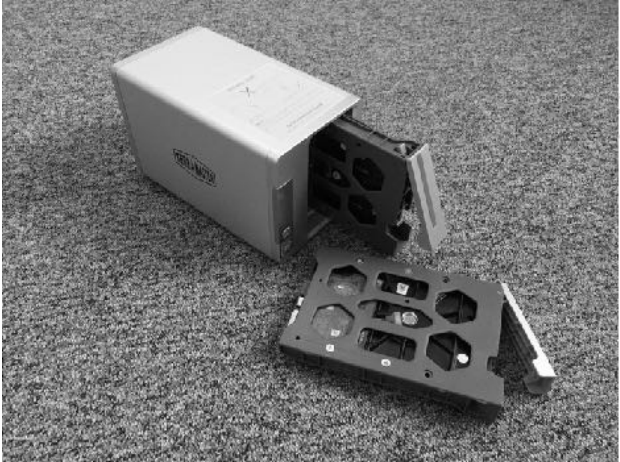
Figure 2: Hard drives being mounted inside a TerraMaster NAS
