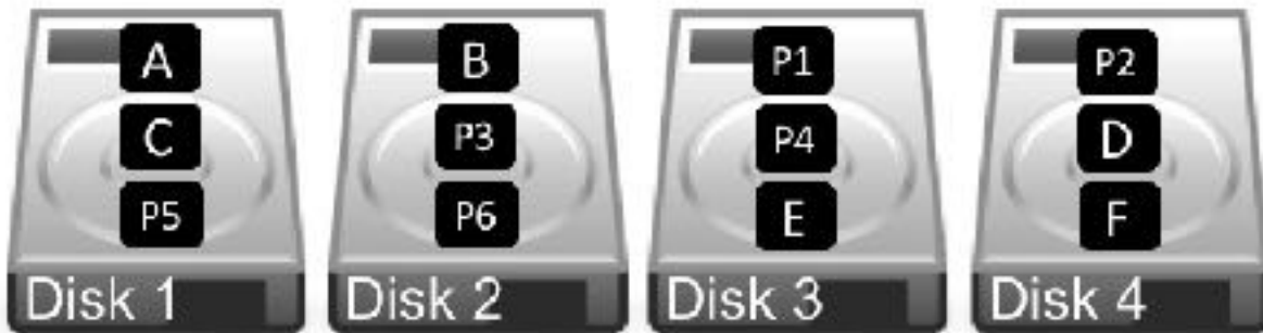
Figure 5: RAID 6 – Multiple drives with double parity information
