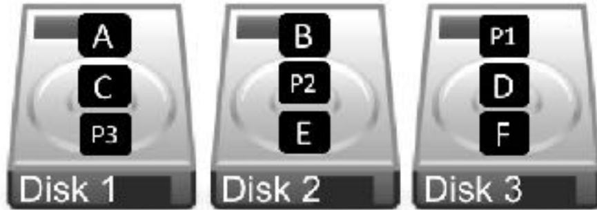
Figure 4: RAID 5 – Multiple drives with parity information
